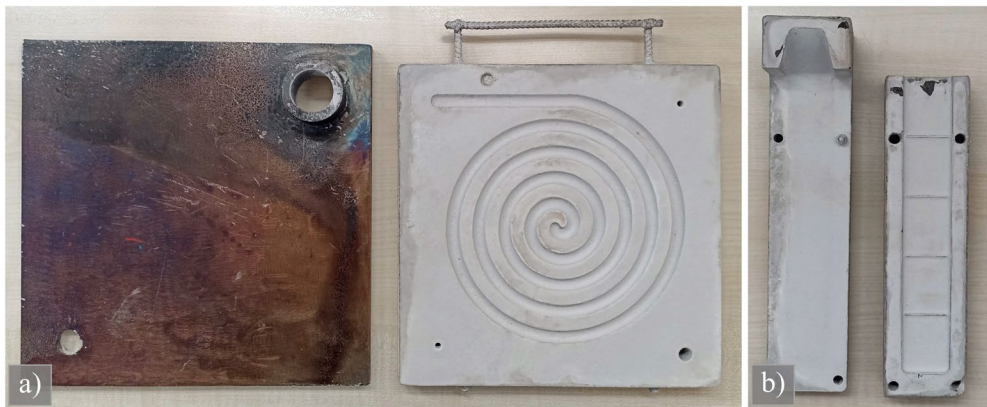
Figure 2. Test moulds; a) Spiral mould, b) K-mold
