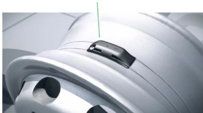
Figure 2. Assembled TPMS sensor on rim
