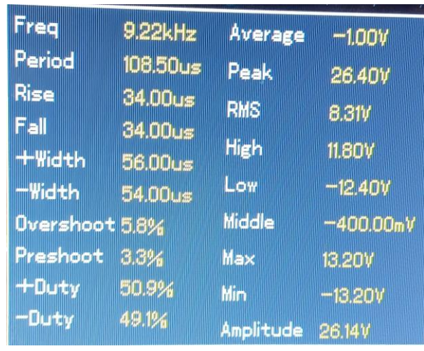
Figure 7. Parameters of the output signal U_{o2cos} of the quadrature RC generator
