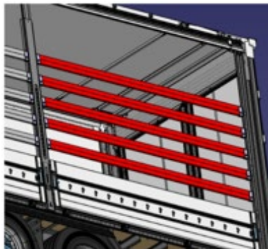
Figure 5. The side profile used during the Code XL annex a test stage
