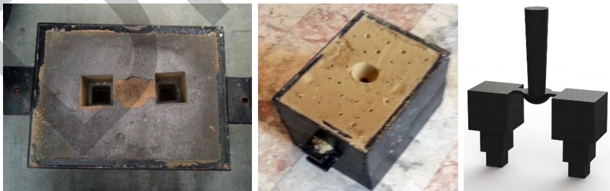
Figure 2. Mould image ready for casting, solid model image after casting
