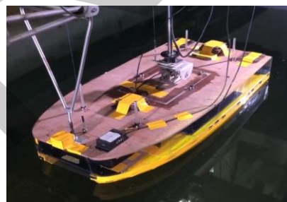
Figure 3. USV Catamaran model setup for resistance test
