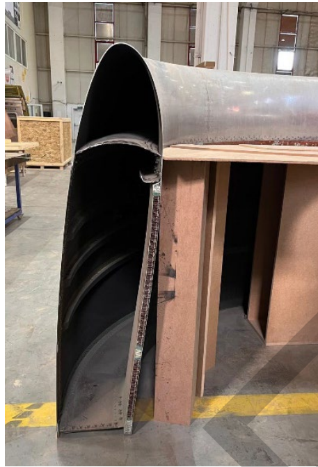
Figure 5. Inside of the cowling
