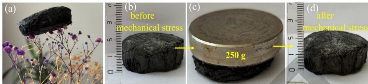
Figure 3. Images showing that MnZn-MOF/GrS (a) is extremely light, (b)–(d) flexible and resistant to mechanical stresses
